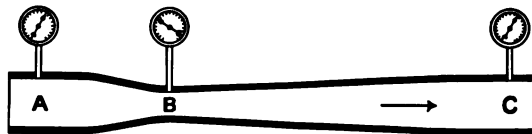
FIG. 318. — Section, Venturi Water Meter.
